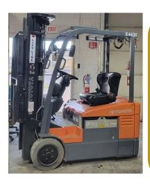
Make: Toyota Model: 7FBEU15 Capacity: 3000 lbs Power: Electric
