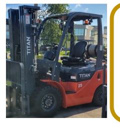
Make: Titan Model: TG25 Capacity: 5,000 lbs Power: LPG Mast: Triple Tires: Pneumatic
