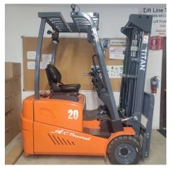
Make: Titan Model: TE2OW3 Capacity: 4,000 lbs Power: Electric Mast: Triple Tires: Cushion
